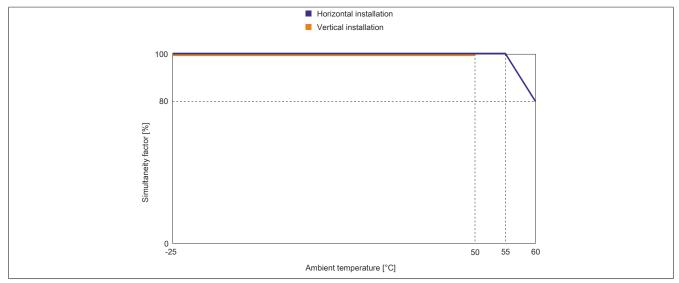
Derating of simultaneity factor at 28.8 VDC input voltage
